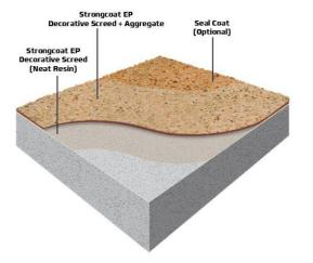
Concrete floors must have a minimum compressive strength of 25 N/mm<sup>2</sup> and a maximum concrete relative humidity of 75% (max. moisture content of 4%), relative humidity can be measured by using hygrometers.
